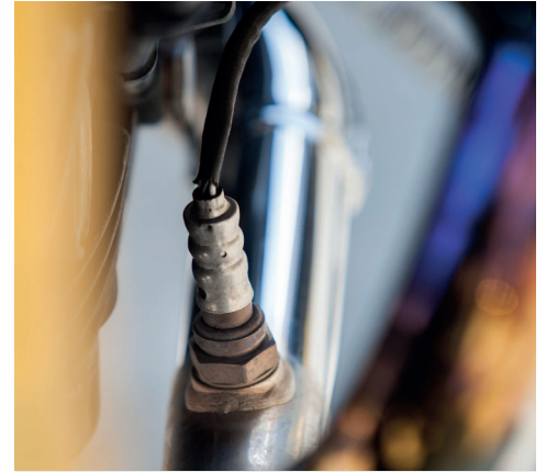
Close-up of a lambda probe
